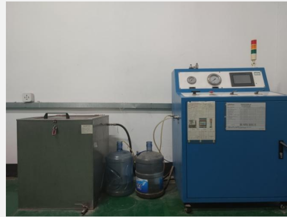
Hydrostatic Test Chamber
