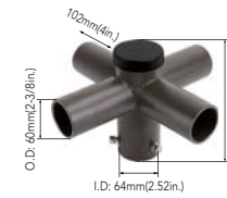
Quad spoke 90° Horizontal Tenon Adapter NO.:R60-SP4-90-D Finish: Dark Bronze Description: Pole mount dual 2-3/8" O.D. tenon, top mount horizontal 90°
