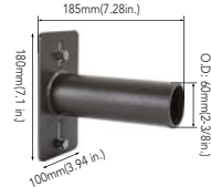
Horizontal Wall and Square pole mount with 2-3/8" O.D. Tenon Bracket NO.:SQ-SP-D Finish: Dark Bronze Description: Wall mount single 2-3/8" O.D. tenon
