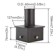
5" Square Pole Mount With 2-3/8" O.D. Tenon Adapter NO.:5SQ-SP-D Finish: Dark Bronze Description: Pole mount single 2-3/8" O.D. tenon, top mount vertical for 5" square pole
